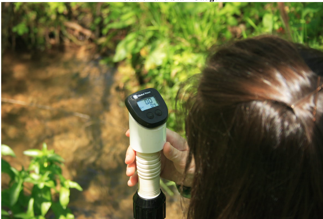
Photo 6: Flow Meter Screen Reading Maximum Velocity
