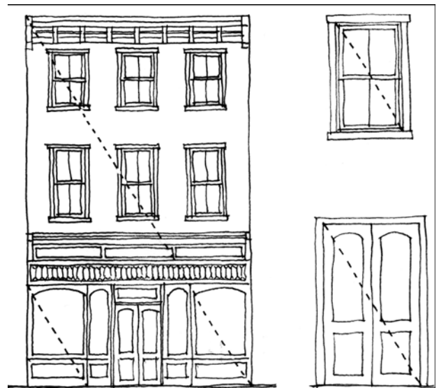
Figure 19. Analysis of three-story commercial building façade showing the repeated proportions in façade elements, beginning with the overall façade and carried down to the proportions of individual glass panes. (Geometrically, when the diagonals of rectangles are parallel, the rectangles are proportional.)
