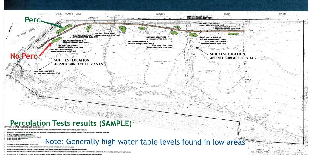
Infiltration rates are a primary determinant for stormwater BMP design
