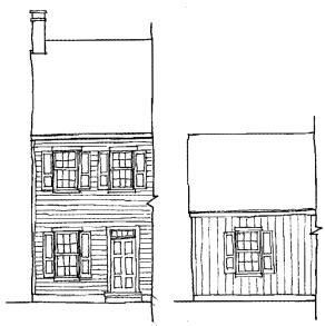
Figure 169 The traditional wood siding for Solebury Township is horizontal clapboarding, while outbuildings may have either vertical-board or horizontal-clapboard siding.
