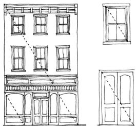
**Figure 128** Analysis of three-story commercial building façade showing the repeated proportions in façade elements, beginning with the overall façade and carried down to the proportions of individual glass panes. (Geometrically, when the diagonals of rectangles are proportional.)
