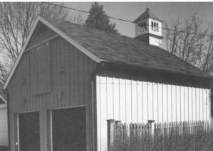
Figure 182 Example of a new garage that is compatible with its historic setting through the use of traditional board-and-batten siding, gabled roof, storage loft, and placement on the lot.
