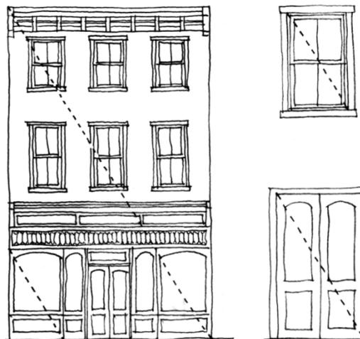
**Figure 128** Analysis of three-story commercial building façade showing the repeated proportions in façade elements, beginning with the overall façade and carried down to the proportions of individual glass panes. (Geometrically, when the diagonals of rectangles are proportional.)
