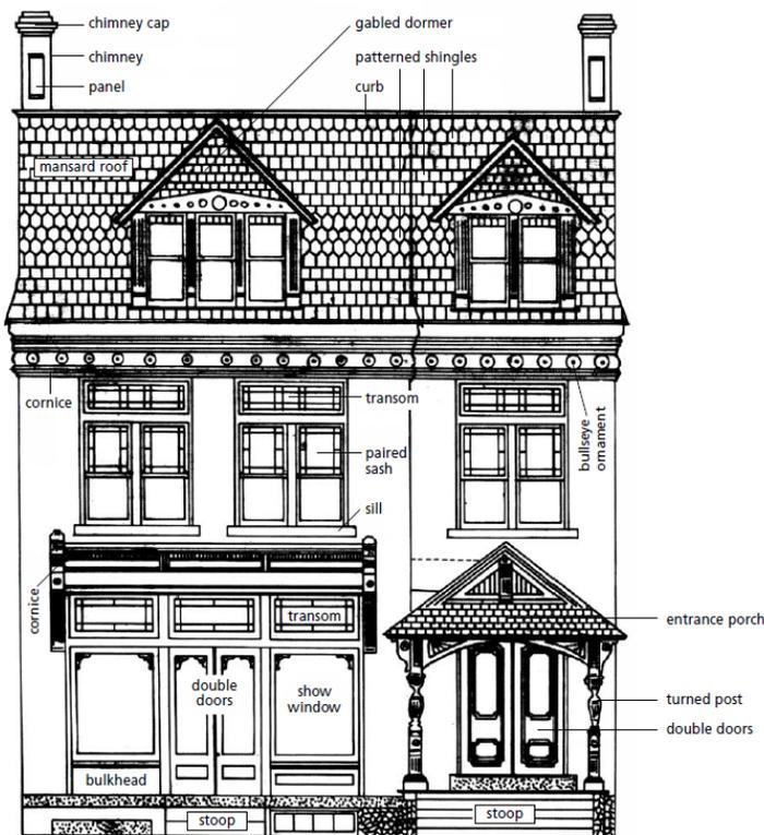
*Figure 68 A house with a patterned slate mansard roof*
